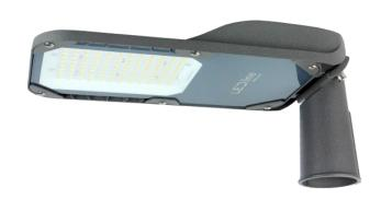
CAMINO 70W road mounting from LED line PRIME is an advanced solution with light performance of 9800 lm. It is characterized by a colour temperature of 4000 K, which provides natural, white light. Made of aluminium and tempered glass, it achieves a high level of protection IP66 and IK08, guaranteeing resistance to atmospheric conditions and mechanical damage. It works in voltage range 220-240 V AC.
