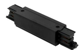
The LUMICANTO bus connector in black with PRIME power supply is a functional solution characterized by a solid design. A product with a length of 163 mm, a width of 33 mm and a height of 32 mm, made of durable plastic. Powered by 220-240V AC voltage and 16A rated current, it provides high reliability. Thanks to the protection class I and IP20 degree, it will be perfect for interiors.
