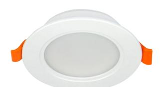
LED line LITE Downlight MOLLY 5W and 500 lumen light stream is a modern solution in a minimalist style. Equipped with SMD LED technology 2835, it provides excellent light efficiency at 100 lm/W. It offers neutral light temperature 4000K and Ra>80 color rendering, which guarantees natural light effect.
