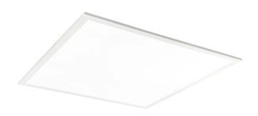
The 34W Backlit PRIME LAW3HAT panel emits a white light with a colour temperature of 4000K generates an impressive luminous flux of 4760 lm, which ensures high luminous efficiency of 140 lm/W. With UGR value<19 guarantees comfortable working conditions, minimizing the glare. The built-in emergency module allows up to 3 hours in case of power outage. Aluminium housing and polystyrene lid material provide an aesthetic appearance and durability.
