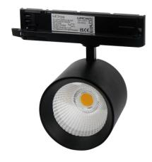
Track light LUMICANTO 6-20W CCT 36/60° in black, is a modern LED line PRIME lighting setting. It uses innovative COB-Bridgelux diodes, characterized by high light performance of up to 110 lm/W and variable colour temperature: 3000 K, 4000 K and 6000 K. The luminaire provides excellent colour reproduction (Ra ≥ 90) and a low flickering factor. With IP20 and IK06 certifications, it offers reliability in different conditions, and its durability is as high as 50,000 hours.
