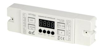
The VARIANTE RF SPI DIGITAL 4in1 (mono/CCT/RGB/RGBW) controller is a modern tool for advanced control of LED strips, offering intuitive operation both directly and using a remote control. Its stable construction is based on an efficient ICP943 circuit, ensuring reliable operation. This model features four output channels and a working frequency of 2.4 GHz, allowing for effective lighting management.
