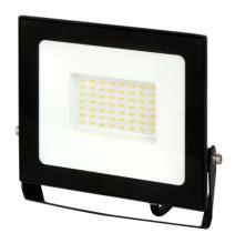
LUMINO 50W LED line LITE is an innovative solution with high light performance of 5,000 lumens at 50 W. Thanks to the colour of the light 4000 K offers natural, white lighting. The product is characterized by IP65 protection class, which provides resistance to dust and water, and IK05 protection level, guaranteeing durability and impact resistance.
