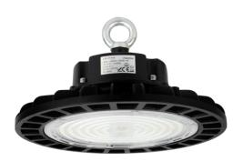
HighBay PHANTOM 190 from PRIME LED line is an advanced lighting solution with a power of 100 W, emitting a light stream as much as 19,000 lm. It is characterized by a light colour temperature of 4000 K and high efficiency of 190 lm/W, which translates into energy savings. Thanks to the IP65 class of tightness and IK08 resistance, the setting is ideal for demanding conditions.
