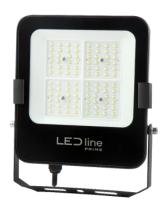
The PRIME Floodlight 30W LED line is an advanced lighting solution with high energy efficiency of 140 lm/W. It emits a luminous flux of 4,200 lumens at a colour temperature of 4000 K. IP66 leak class guarantees resistance to difficult weather conditions, making it ideal for external applications.
