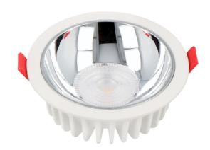
LED line downlight 15W 1500Im 4000K QUANTUM is a modern light source with high energy efficiency, which provides a light stream of 1500 lumens. The use of COB LED technology allows to achieve excellent light performance of 100 lm/W and Ra colour rendering coefficient of 85, which guarantees natural color reproduction. The housing is characterized by a nominal power of 15 W and a 60° light distribution angle.
