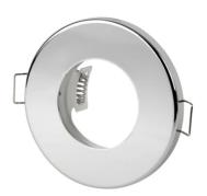
LED line ceiling housing Prime combines modern design with functionality, offering elegant round shape and chrome finish. Its diameter is 85 mm and the dedicated light source has a diameter of 50 mm. Made of transparent glass and powder-painted sheet metal, it provides not only aesthetics but also durability. With IP44 protection class is resistant to moisture.
