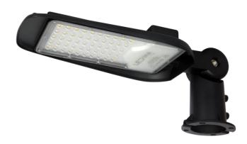
STREETLITE 50W road luminaire is characterized by high light efficiency of 100 lm/W and a total light stream of 5000 lm. Its housing made of durable aluminium casting provides effective heat discharge, which extends the life of LEDs to 36,000 hours. Polycarbonate cartridge guarantees IP65 seal class and IK08 impact resistance.
