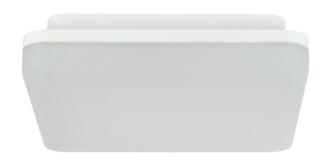
ACTON 18W LED Plafon is a modern lighting setting with high light efficiency of 1900 Im and 3000 K colour temperature, providing pleasant, warm light. It is characterized by IP54 leak class and IK08 resistance, making it ideal for use under difficult conditions. The reliability of the product is underlined by the five-year guarantee. Polycarbonate housing guarantees durability and aesthetics.
