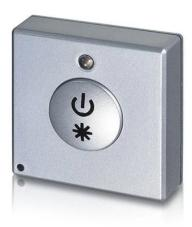
LED dimmer RF Sunricher Pilot MONO is an advanced wireless controller dedicated to precise lighting management. It offers a unique dimming function in the range from 0.1% to 100%, allowing smooth brightness adjustment without flickering effect. Thanks to the logarithmic dimming system and the range of operation up to 20 meters, it provides stable and comfortable use.
