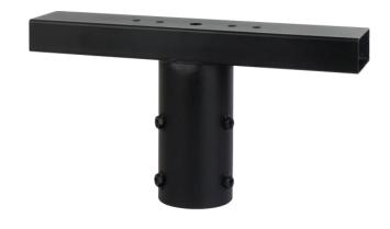
The light holder for the folding lighting pole is dedicated for installation on poles with a diameter of 60 mm, allowing direct installation of the lamp. It has a mounting hole spacing from -7.5 cm to +7.5 cm, allowing versatility in use with PRIME models with a maximum power of 200W. The mounting base dimensions are 40x8 cm, providing a stable and robust design.
