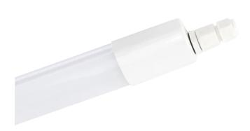
LINIX 36W 4000K 4320lm IP65 LITE from LED line LITE is a modern lighting solution, characterized by high light performance of 4320 lumens. At 36 W power consumption and 220-240 V AC power supply, the product achieves an excellent PF power factor of 0.95. Thanks to the IP65 class of tightness and IK07 strength, the housing is resistant to adverse weather and mechanical conditions.
