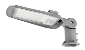
STREETLITE 100W road luminaire from LED line LITE is characterized by a solid housing with high quality aluminum, which ensures excellent heat draining and longevity of LEDs. Thanks to the IK08 parameters, it is resistant to mechanical damage, and the polycarbonate canister provides IP65 protection against dust and moisture. It emits a luminous flux of 10,000 lm at 100 lm/W light efficiency and 4000 K colour temperature.
