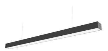
LED line mount PRIME FUSION 40W 4000K is a modern product with a high light efficiency of 130 lm/W, providing a light stream of 5200 lm. Made of durable aluminum, it guarantees excellent heat draining and long service life, reaching L70B50 of 50,000 hours. IP20 and IK08 leak class provide adequate protection against external damage.
