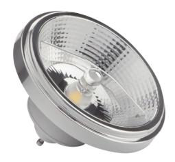
LED line ES111 is an advanced 12W lamp, offering an impressive light stream of 1080 lm. It is characterized by a neutral colour of light 4000 K, which provides comfortable lighting in each interior. It is powered by 230 V AC alternating current and has a light performance of 90 lm/W. Thanks to an angle of 45°, it is ideal in spaces where precise illumination is required. The product has a long shelf life of up to 50,000 h.
