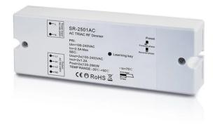
Sunricher TRIAC 1.2Ax2 230V receiver is an advanced triac dimmer designed to work at 100-240VAC voltage. It has two channels, each with a maximum load of 1,2 A, which provides flexibility in lighting applications. Equipped with a modern RF interface, it allows you to work with Easy RF pilots and support push dim function when connected to the switch.
