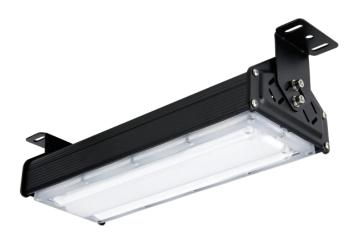
LED STREAKBAY High 50W Bay and 5000 Im light stream is a modern lighting solution that is characterized by high performance, reaching 100 Im/W. Thanks to the colour temperature of 4000K and the asymmetric lens 120x60°, it provides even illumination for large spaces with minimal light scattering. Made of solid cast aluminium housing and high degree of protection IP65 guarantee resistance to difficult operating conditions.
