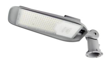
STREETLITE LED line LITE 150W is an advanced lighting solution that is distinguished by a high-quality aluminium housing for excellent heat removal. It is characterized by a high luminous efficiency of 100 lm/W and a total luminous flux of 15000 lm. Thanks to the IP65 protection degree, it is resistant to dust and moisture, and the IK08 resistance class protects against mechanical damage.
