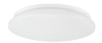
LED Line LITE with 12W power and warm colour temperature 3000K provides a light stream of 900 lumens. Thanks to the IP44 leak class, the product is resistant to moisture, making it suitable for different locations. The 260 mm round housing ensures a uniform scattering of light in an angle of approximately 120°. Ra≥80 color rendering rate guarantees natural color reproduction.
