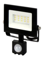
LED LUMino 10W LED line LITE is an ideal combination of efficiency and modernity. It offers a light stream of 1000 lumens at 4000K light colour temperature, providing a neutral and pleasant atmosphere. Thanks to the use of the PIR motion sensor, the device automatically switches on when motion is detected, which significantly reduces energy consumption.
