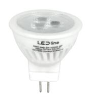
LED light bulb MR11 3W by LED line PRIME is a modern light source with a luminous flux of 330 lm and a colour temperature of 4000 K. It is characterized by high light performance at 110 lm/W and a wide range of power supply voltages from 10 to 14V AC/DC. The 38° light angle provides precise lighting. Ceramic housing guarantees durability, and low flickering rate and high colour rendering rate Ra ≥80 provide comfort of use.
