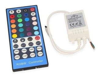
RGBW IR 12V 8A LED controller is an advanced device dedicated to precise LED lighting control. It uses PWM (Pulse Width Modulation) technology, which allows for smooth changes in brightness and color of light. Supports RGBW LED tapes, allowing to create various light effects. Control is done by means of an infrared remote control with 40 buttons, which ensures comfort of use.
