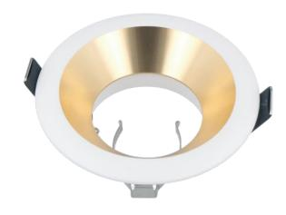
The LED line OLTIKA ceiling housing in an elegant white and gold finish combines aesthetics with functionality. Made of high quality aluminium casting, it has a diameter of 100 mm and IP20 leak class, which allows it to be used inside buildings. With a maximum power of 35W and the ability to adjust the direction of illumination, it provides optimal lighting. Easy installation in a 75 mm hole allows for quick installation of fittings in different interiors.
