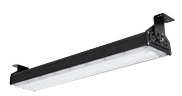
HighBay STREAKBAY from a 100W LED line LITE and a 10,000 lm light stream is a perfect solution for demanding industrial environments. It is characterized by colour temperature 4000K, which provides natural color reproduction. Its construction from aluminium casting in IP65 protection class guarantees resistance to difficult weather conditions.
