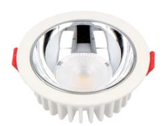
LED line mounting downlight 7W QUANTUM is an innovative lighting solution with high performance. Thanks to the use of the Bridgelux COB diode, it generates a light stream of 700 lumens at a power of 7 W. Neutral colour of light 4000 K favours natural light. The high colour rendering rate Ra 85 provides faithful color reproduction, which is crucial in precise applications.
