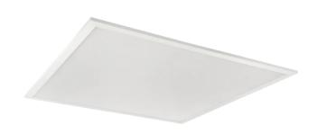
The PRIME Backlit LED line panel with 34W and 4000K color temperature is an ideal solution for demanding applications. By generating a luminous flux of 4,760 lumens, it provides efficient and energy-efficient lighting, achieving a capacity of 140 lm/W. Thanks to the low brightness index UGR<19 and the high quality of aluminum and polystyrene, this product is distinguished by durability and comfort of use.
