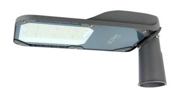
CAMINO 50W LED line PRIME is an innovative lighting solution that stands out with a power of 50 W and a light stream of 7000 lumens. Thanks to high light efficiency of 140 lm/W and the use of LUMILEDS LEDs, it guarantees reliable operation. It offers neutral colour temperature 4000 K and IP66 leak classification provides resistance to adverse weather conditions.
