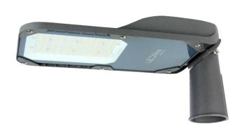
CAMINO road luminaire from LED line PRIME is an innovative 50W solution that emits as many as 6500 lumens with high light efficiency of 130 lm/W. The LUMILEDS used LEDs guarantee reliability and long life up to 100,000 hours. The warm-colour light version (3000K) creates a pleasant atmosphere. Resistant to extreme conditions, it is characterized by the degree of protection IP66 and IK08, which ensures durability of materials: aluminium and tempered glass.
