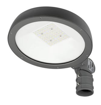
The PRIME Elida 70W LED line housing is an excellent example of the combination of performance and elegance. Offering a light stream of 8400 lm and high efficiency of 120 lm/W, it provides excellent lighting at 4000 K colour temperature. Made of aluminium casting, it is characterized by resistance to atmospheric conditions (IP65) and impaction IK08. Thanks to LED technology, Elida guarantees longevity, reaching life of up to 50,000 hours.
