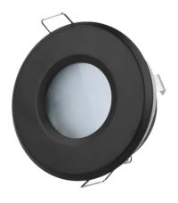
The LED line Prime ceiling setting offers modern solutions in indoor and outdoor lighting. It is characterized by elegant design thanks to a matt glass lens and a solid aluminium cast housing, which ensures durability and aesthetics. It has IP44 seal class, which makes it resistant to moisture. It is easily mounted in holes with a diameter of 73 mm and the application of adjustment of the angle of light increases functionality.
