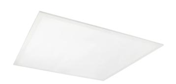
The PRIME 25W LED line panel is an innovative 595x595 mm ceiling luminaire, characterized by high quality workmanship and even light distribution. Thanks to the use of SMD LEDs 2835, the panel generates a light stream of 4000 lm at 160 lm/W efficiency. The light colour is 4000 K, providing neutral lighting. The housing guarantees a longevity of 50.
