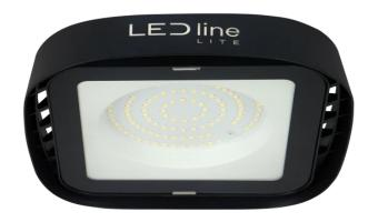
LED line LITE HIGH-BAY ECOBEAM with a power of 100W and a light stream of 10000 lumens is characterized by excellent energy efficiency of 100 lm/W. Its colour temperature is 4000K, which provides neutral, eye-pleasant light. Made of aluminium casting and tempered glass, the housing achieves IP65 protection, guaranteeing resistance to dust and water.
